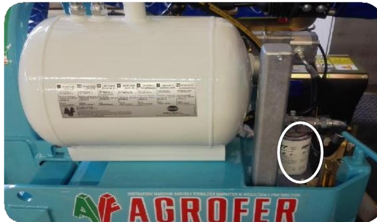
Picture 20 – Oil level, tank and oil filter check
