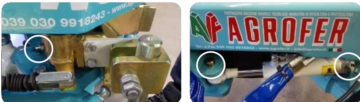
Picture 18 – Greasing points “Feeler pin cylinder”
