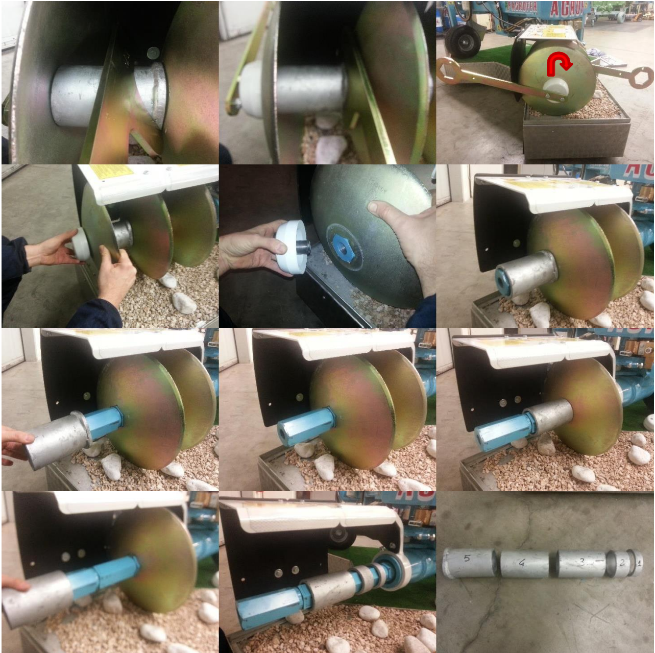
Picture 11 – Dismantling phases disk assembly
