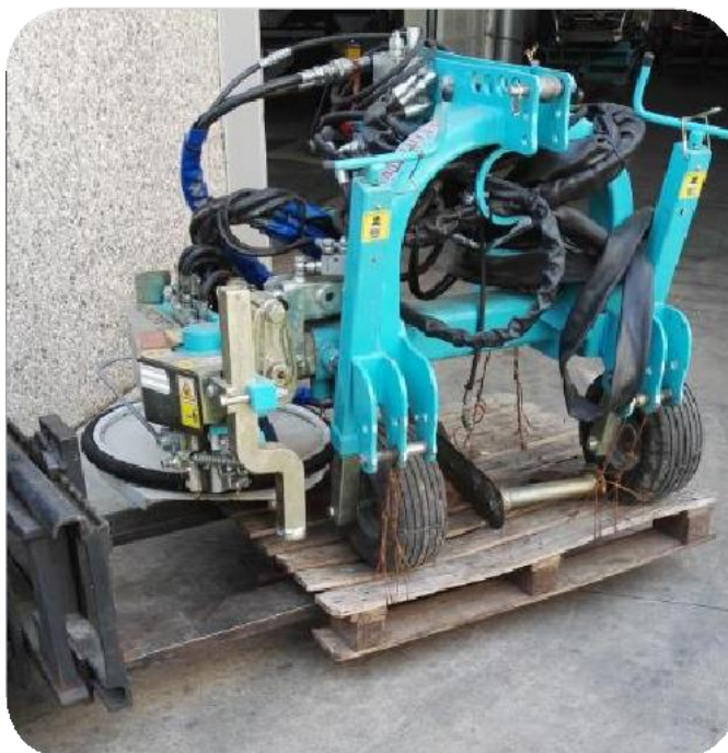
Picture 4. Position of the blades of the forklift to move the machine delivered with packaging.
