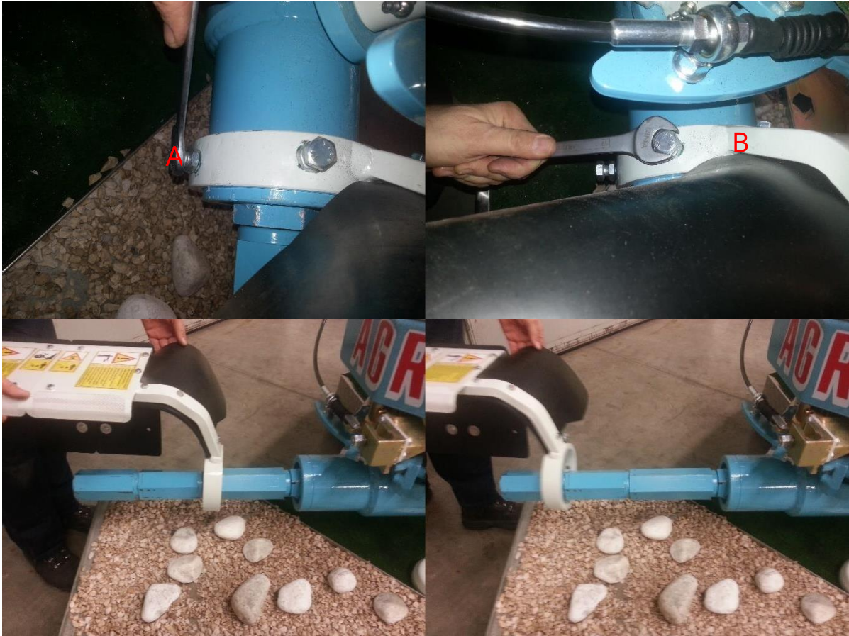
Picture 12 – Dismantling disks casing
