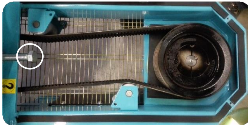
Picture 21 – Register for regulating the tension of the trapezoidal belt
