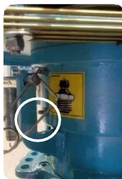
Picture 19 – Greasing points “Slewing baring under sheave”
