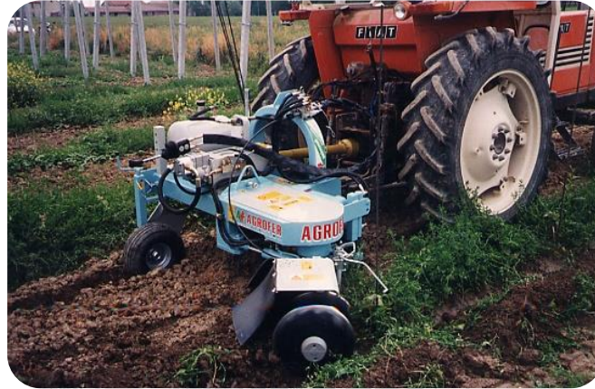
Picture 2. Baring / ridging machine working
