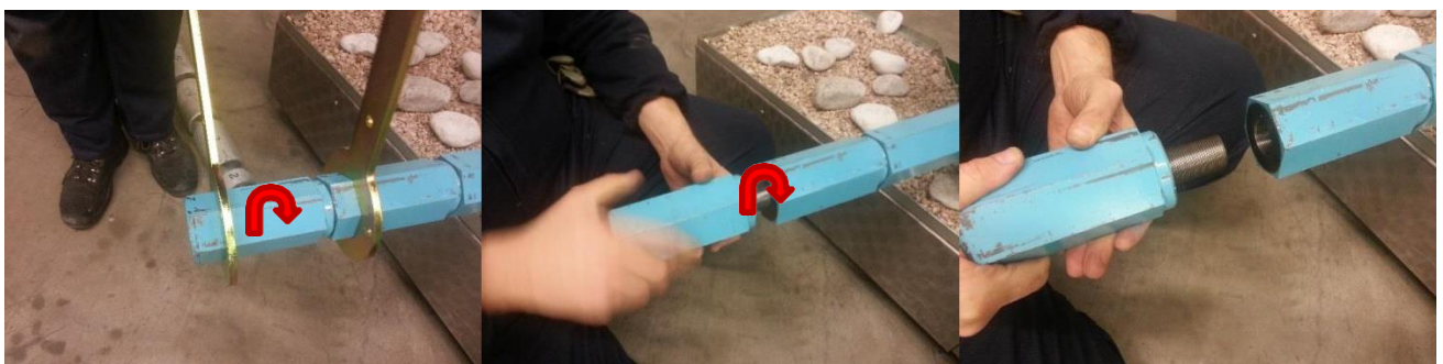
Picture 15 – Removing the 3° module disk holder
